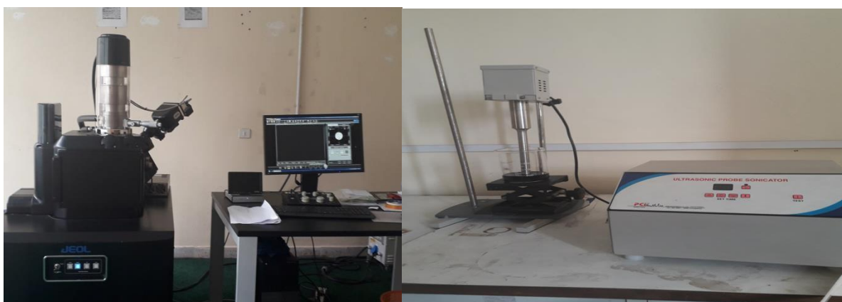
Figure A 0-2: (a), Scanning Electron Microscope (b) Probe horn sonicator at 50% amplitude power
