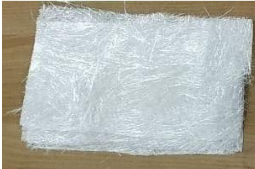
Figure 3.2 Commercial E-glass fiber
