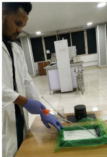
(e) impregnating epoxy resin with roller
