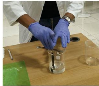
(b) Epoxy-hardener mixing
