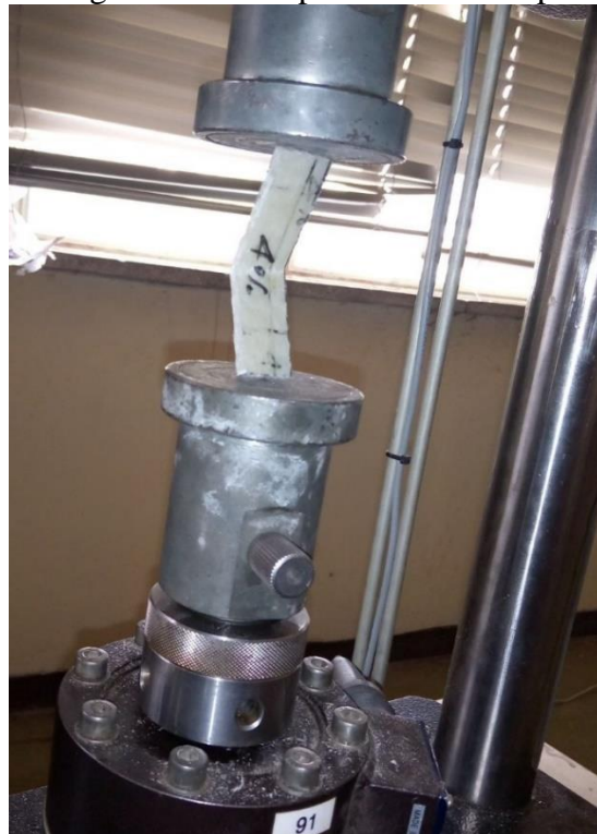
Figure 3.24 Compression test specimen at fracture
