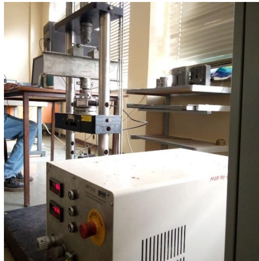
Figure 3.16 Gunt Hamburg WP 310 hydraulic material testing machine
