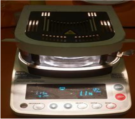
Figure 3.7: Instant moisture analyzer
