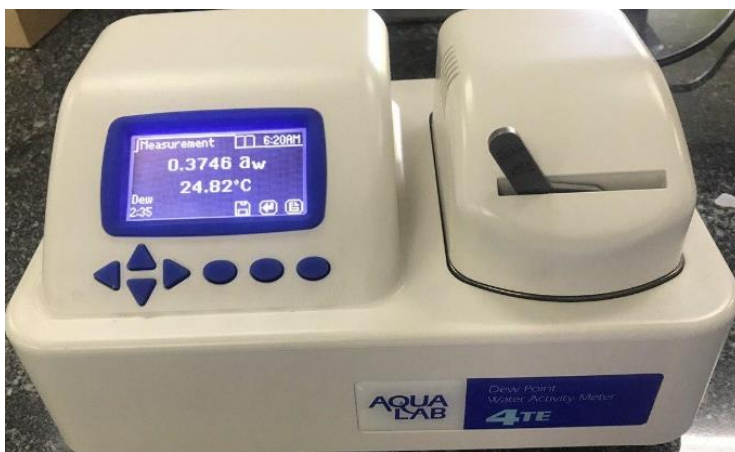
Figure 3.9: Water activity meter used in the research work.
