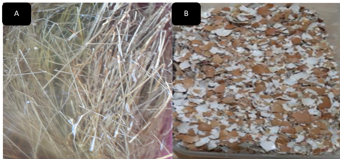
Figure 3.3 (A) Flax fiber retting and soaking process and (B) Eggshell particles
