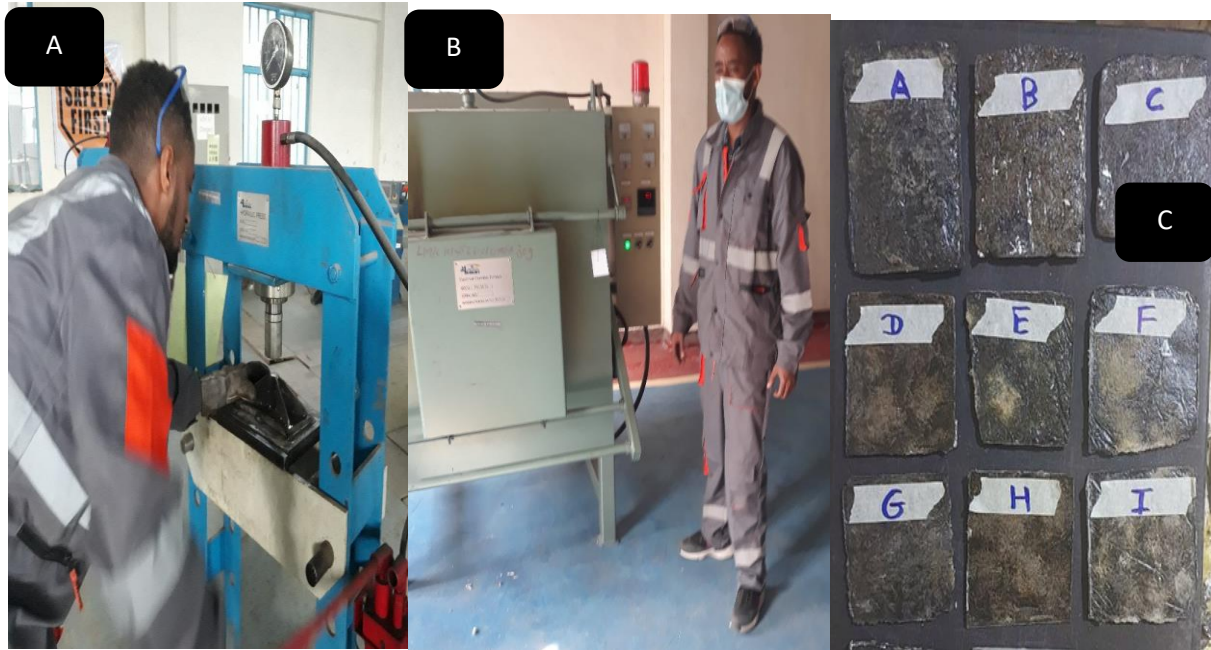
Figure 3.9 (a) Press machine settings (b) curing process (c) Samples of brake pad
