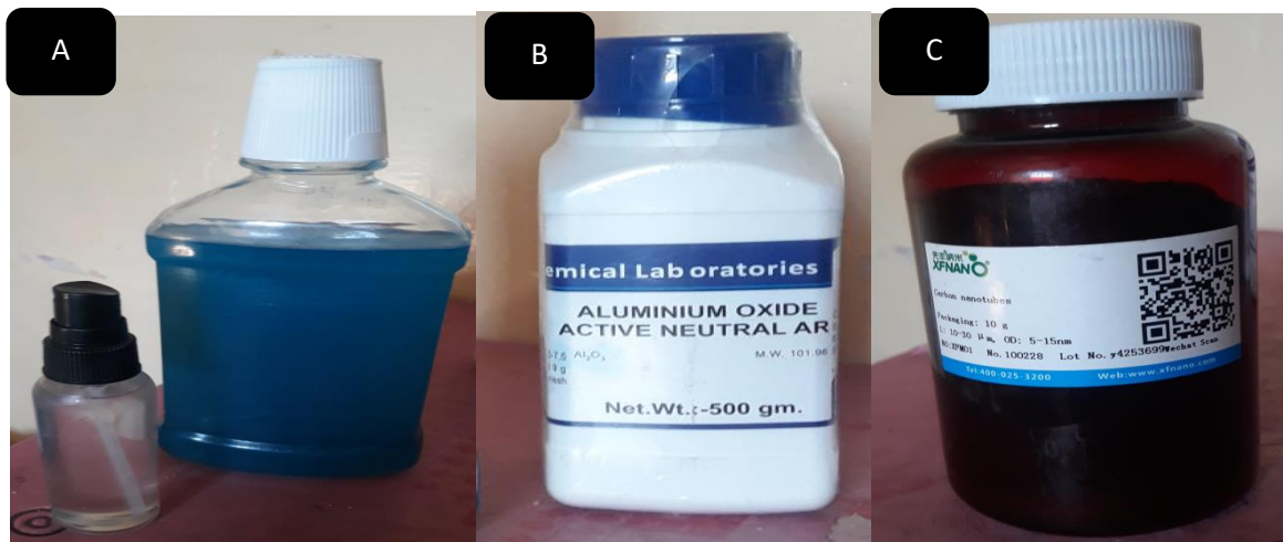
Figure 3.6 (A) polyester resin & hardener,(B) Al_2O_3 , and (C)MWCNTs
