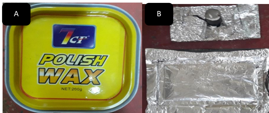
Figure 3.8 (a) Wax and (b) Aluminum foil sheets as a releasing agent
