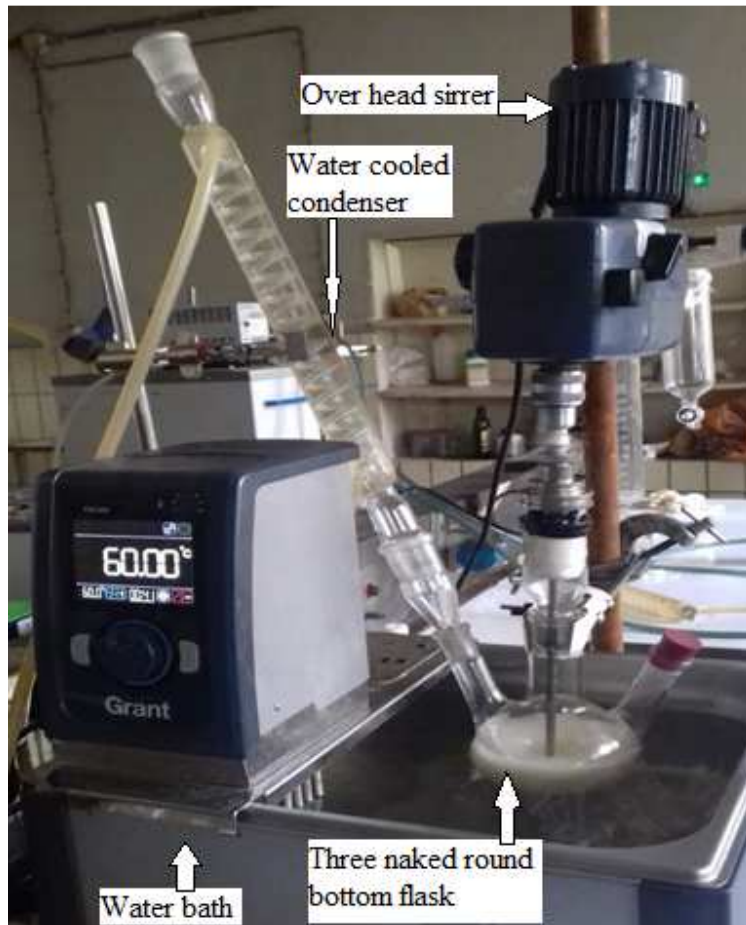
Experimental setup for a two-step acid-base catalyzed transesterification reaction
