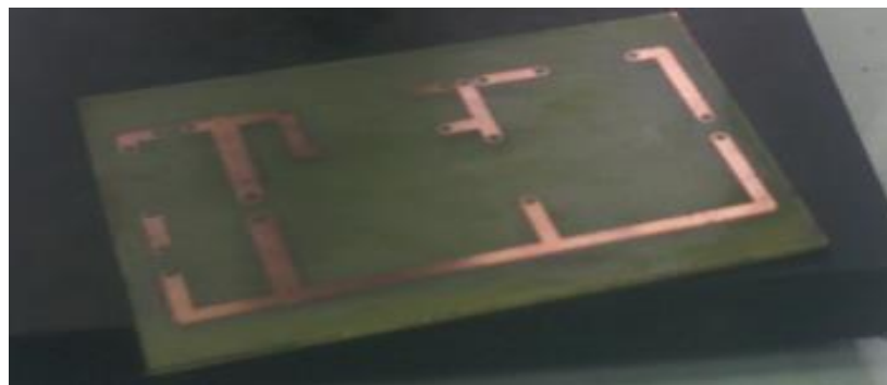
Figure 3.6 Etching the plate
