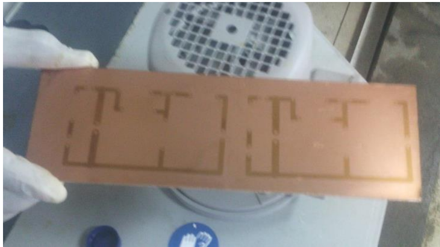
Figure 3.5: Transferring PCB layout in to photo sensitive material
