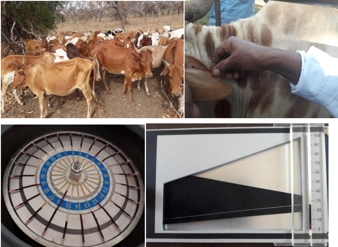
Figure 2. Animals congregated for bleeding (upper left), bleeding of animals (upper right) Micro-haematocrit tube after centrifugation (lower left) and PCV reading (lower right)
