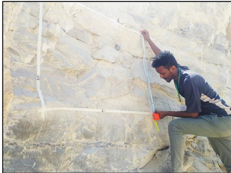
Figure 10.1 1m Volumetric count of an exposed rock face in the study area.
