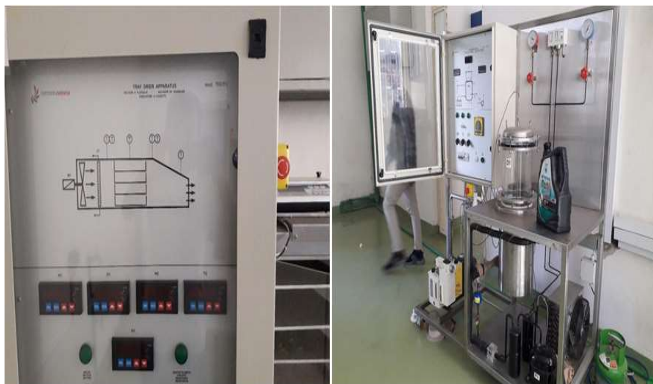
Figure B-10 Tray and Freeze drying apparatus
