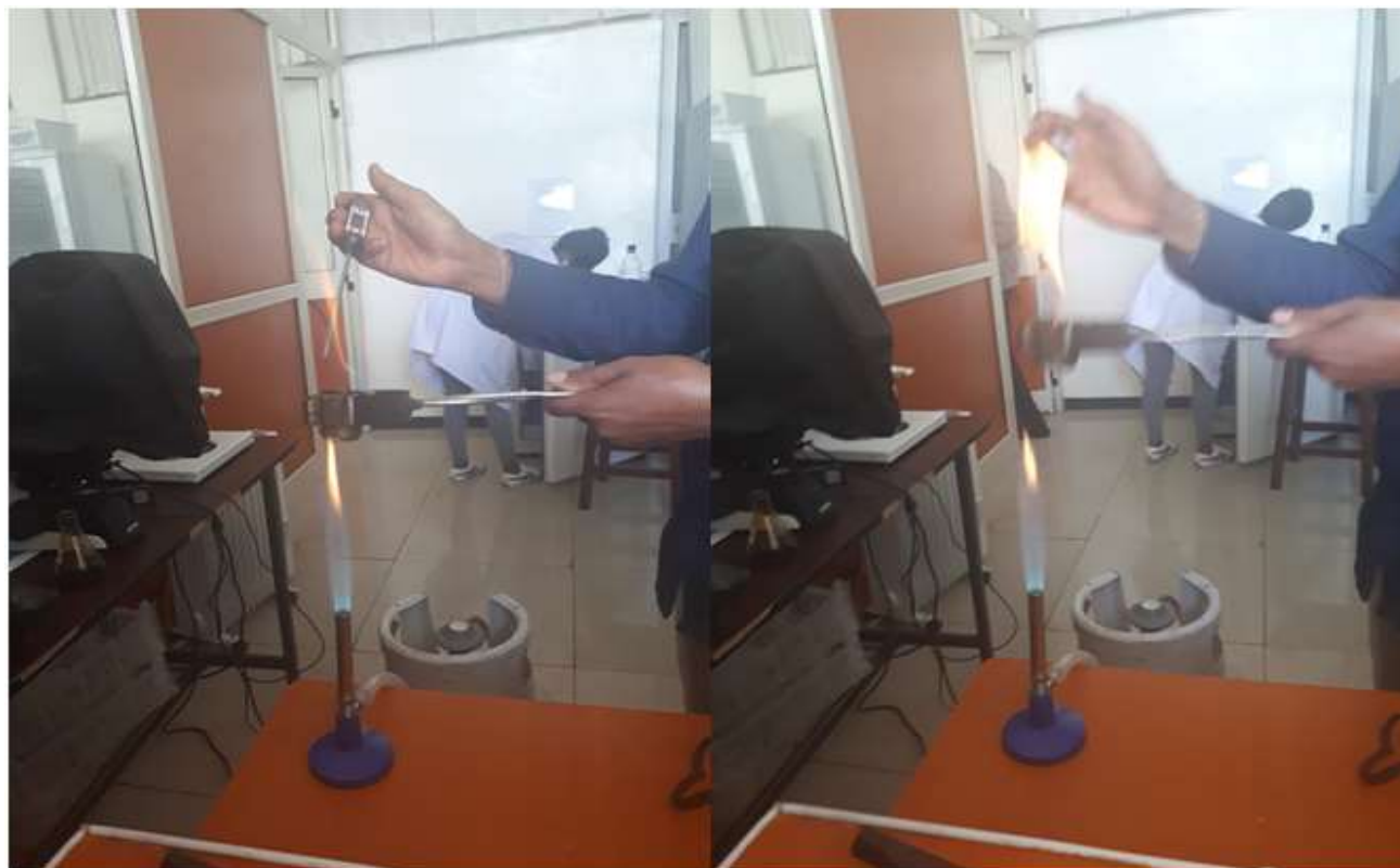
Figure B-9 Flash point determination
