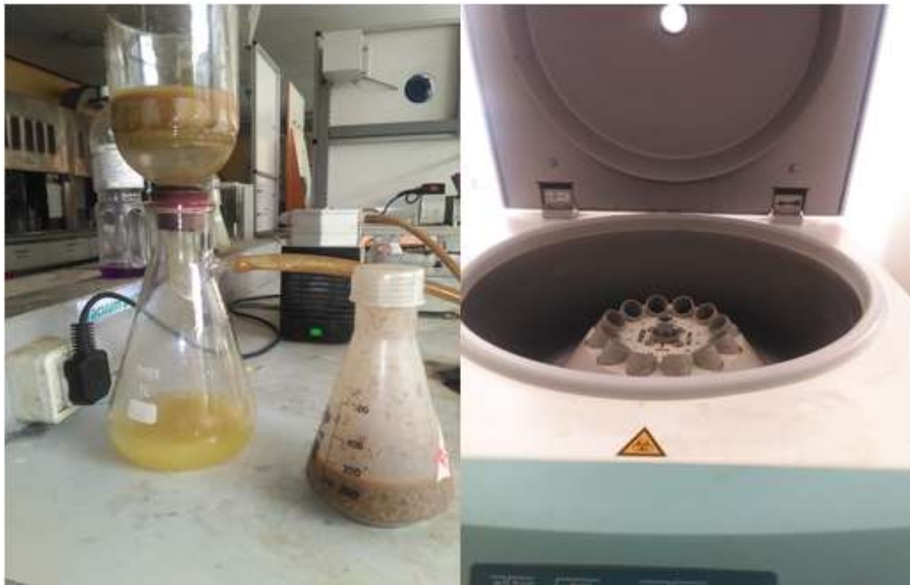
Figure B-5 Filtration and centrifugation of the extract
