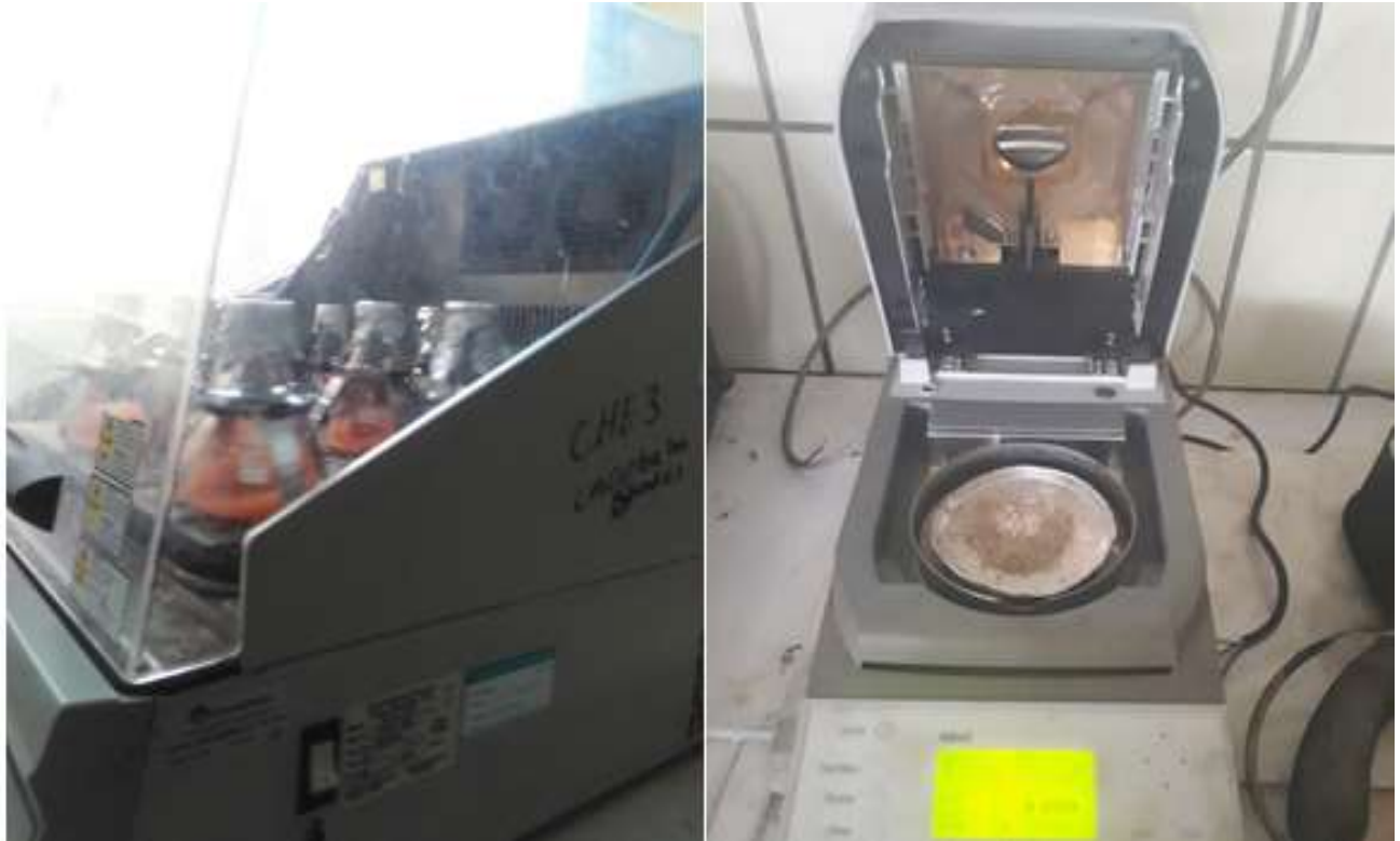
Figure B-11 Shaker incubator and Moisture content analyzer
