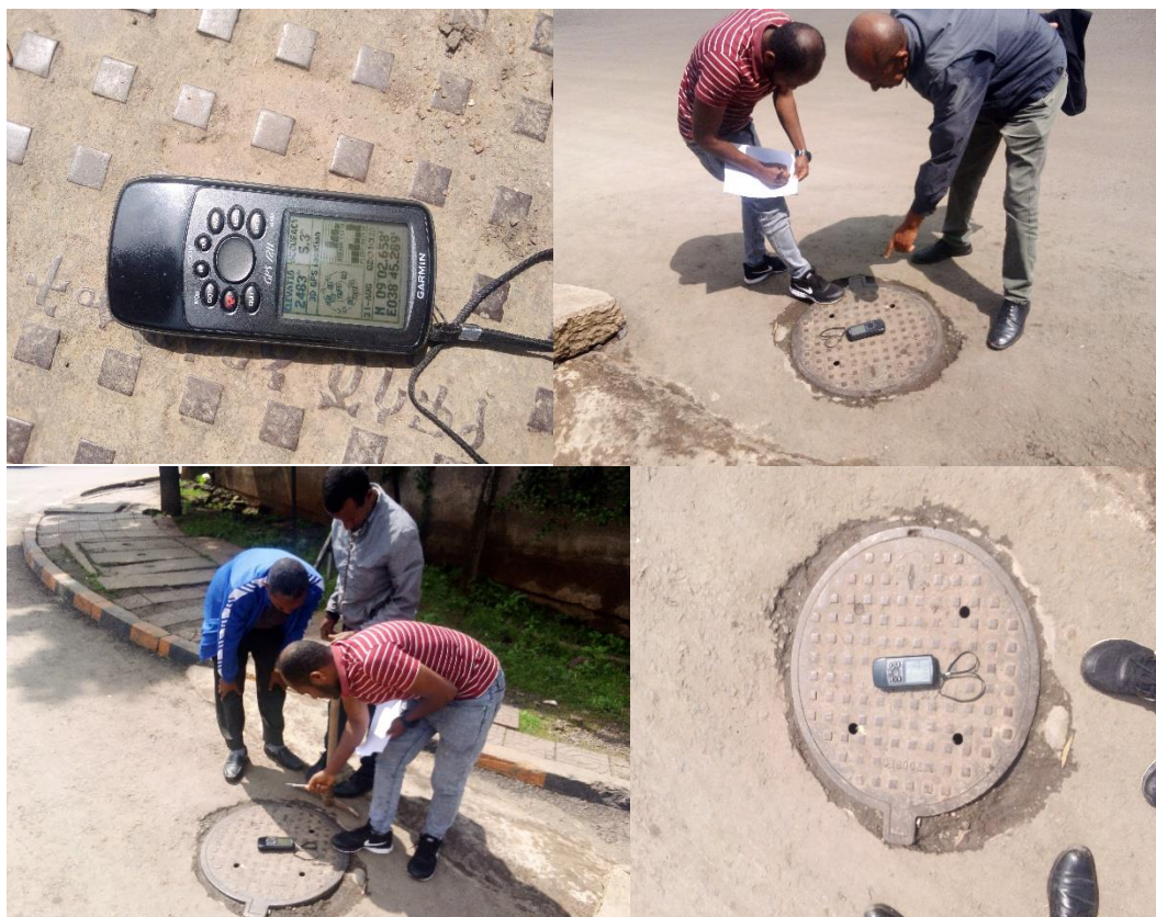
Figure 3: 17 measuring ground elevation and X, Y coordinates
