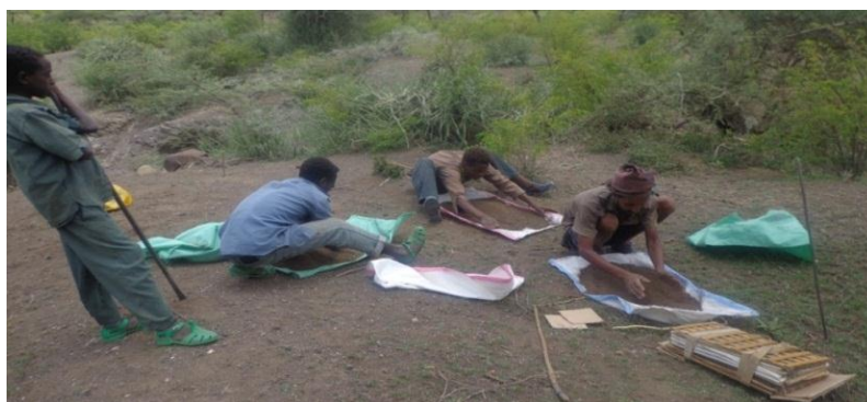
Workers mixing the soil samples
