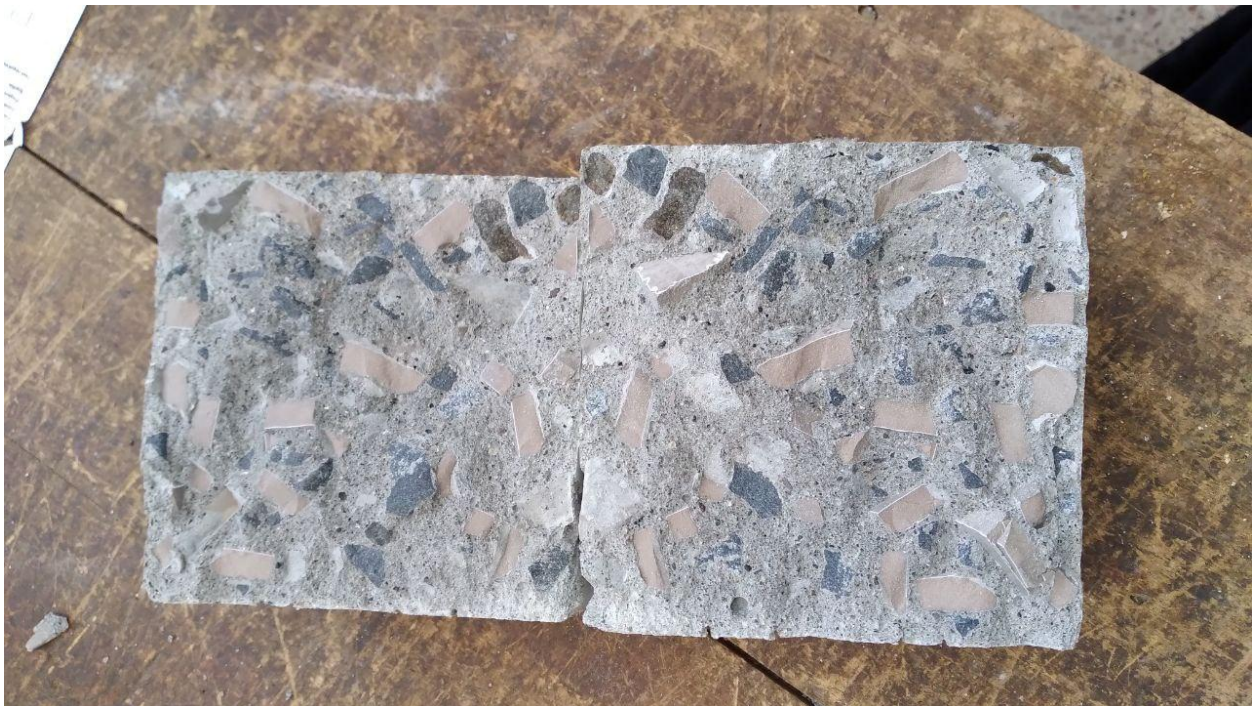
Pictures of the concrete mix 30% and 40% replacement of ceramic aggregate(inside)
