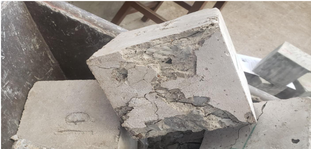
Pictures of the compressive test, and cubes after the test the first cube being at room temperature and the later being after exposed to high temperature
