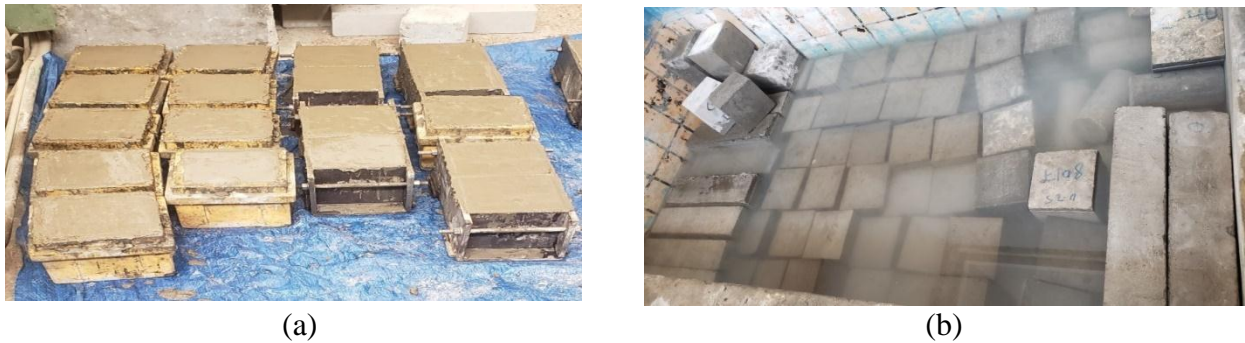
Fig 12.(a) concrete mix in mold (b) curing specimens
