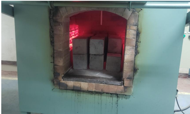
Fig 13. concrete cubes in furnace under high temperature
