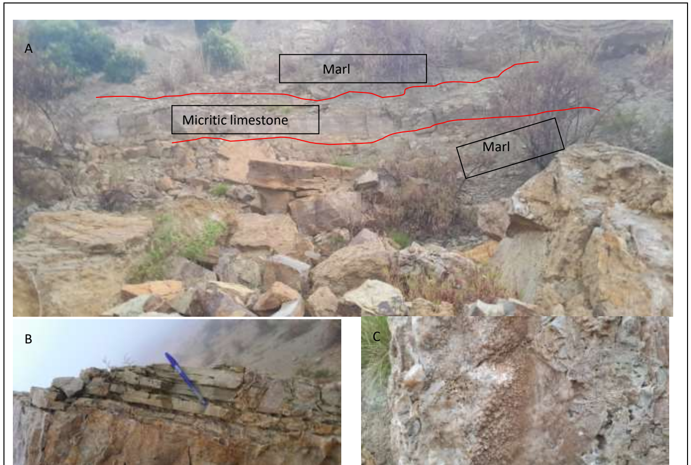
Figure 4. 2: Marly limestone from S1K1 A, above and below the red arrow are pure Marl and between them is Micritic Limestone B, Marly Limestone, C, calcite precipitated in Marl (later precipitated)
