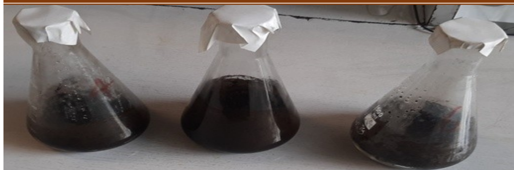
Fig.3.2: Carbonized EL powder soaked in H_3PO_4
