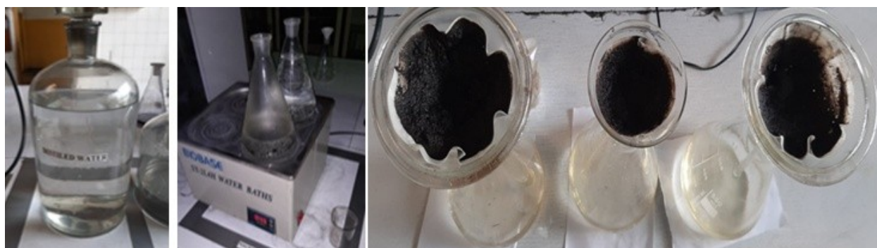
Fig. 3.3: Filtration of soaked Enset leave using hot distilled water
