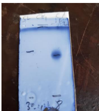
Figure 7: TLC profile of fractions of CH:EA extract of the Stem Bark of S. longipedunculata
