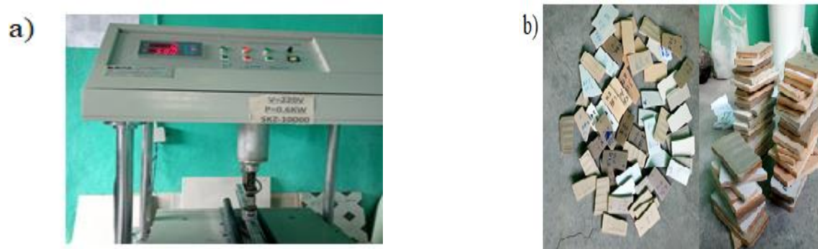
Figure 3.6: Fired strength analysis a) MOR testing machine b) glazed and unglazed samples.
