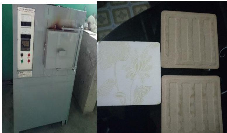
Figure 3.5: Electrical kiln firing at 1000, 1100 and 1200°C and the products for 2 hours
