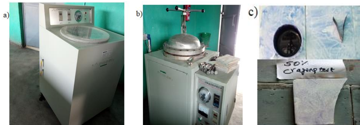
Figure 3.8: a) Water absorption machine b) Crazing Test Machine/Autoclave, c) crazed tiles
