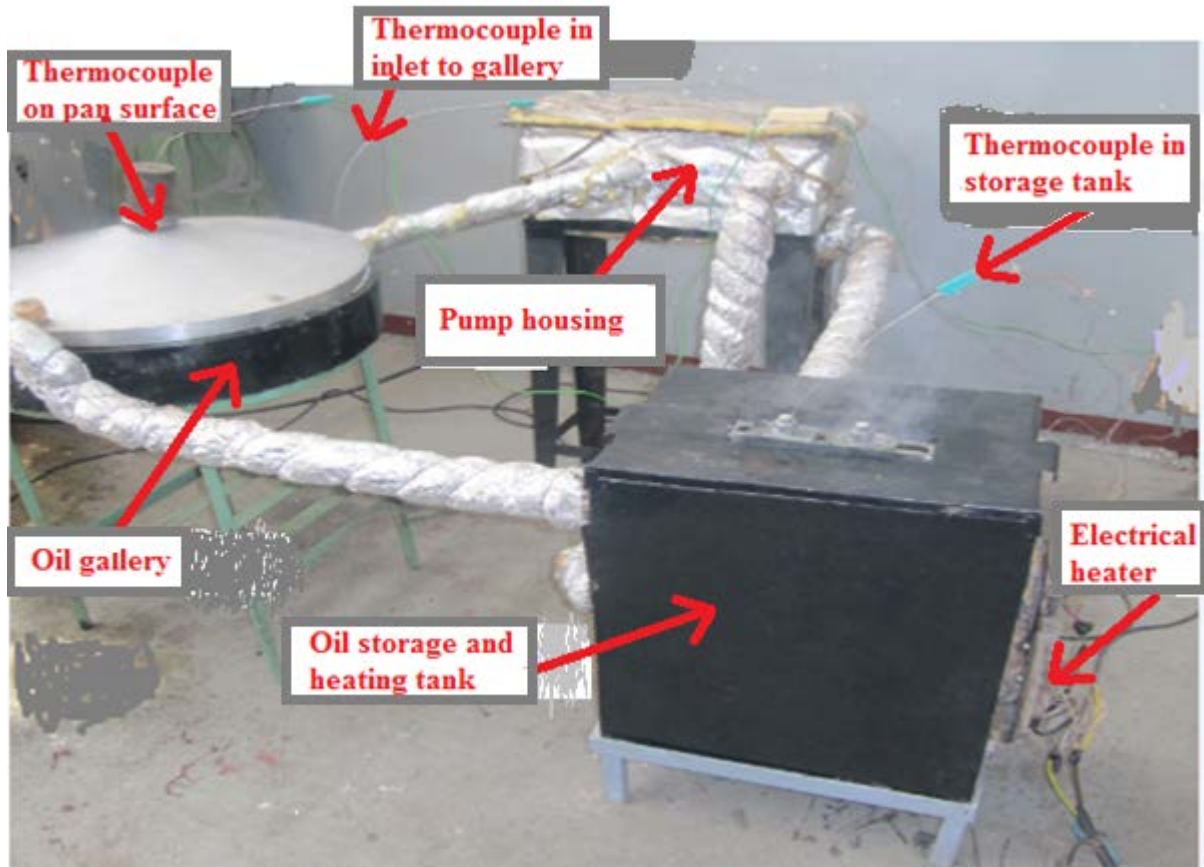
Figure 5.1: Main components of the laboratory model and thermocouples inserts during experimental test
