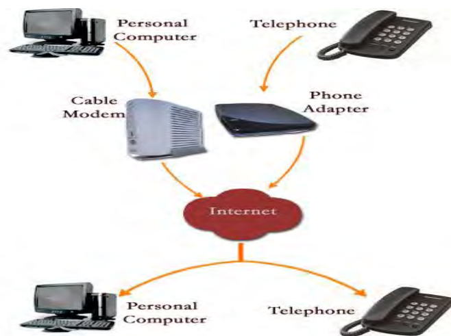
Figure 1. Simplified VoIP infrastructure
