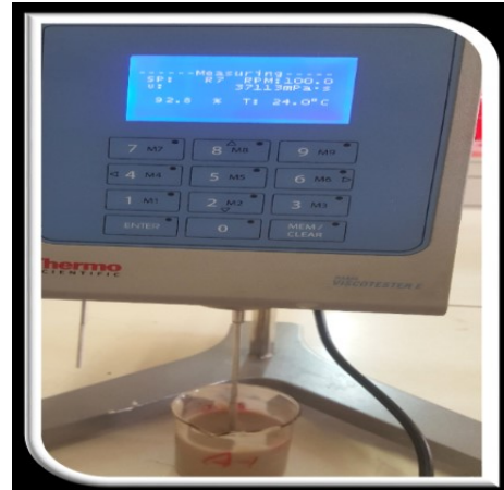
Figure 2.4: viscosity measurement of teff batter ready to bake during the work
