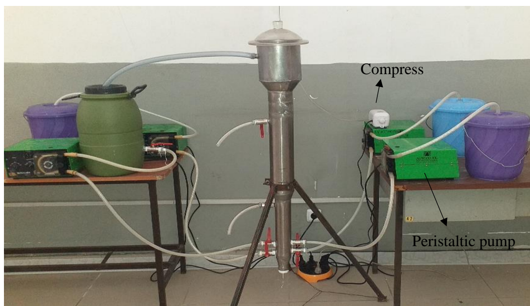
Figure 3.2 Laboratory scale struvite crystallization system.
