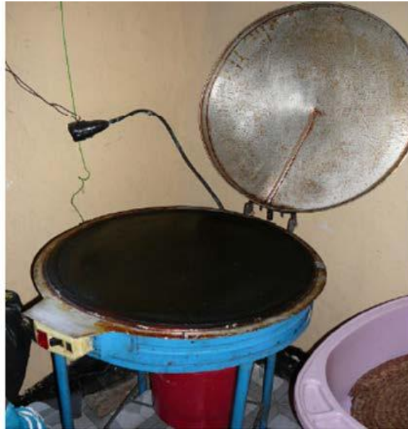
Figure 2.3 Electrical Injera baking Method
