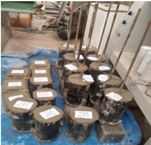
Figure 3.12. Concrete Specimens after casting
