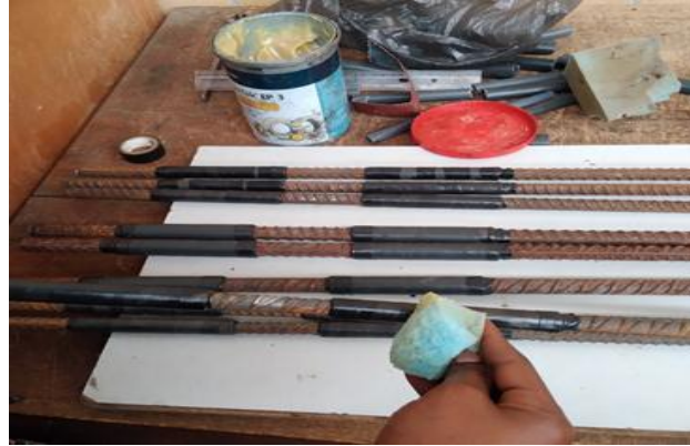
Figure 3.6. Painting of Machine grease on External surface of PVC tube
