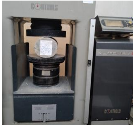
Figure 3.15. Test setup of Splitting tensile strength test
