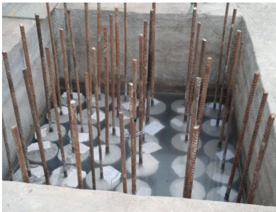
Curing of concrete member specimens
