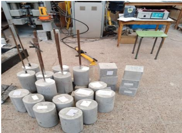
Pullout bond strength test
