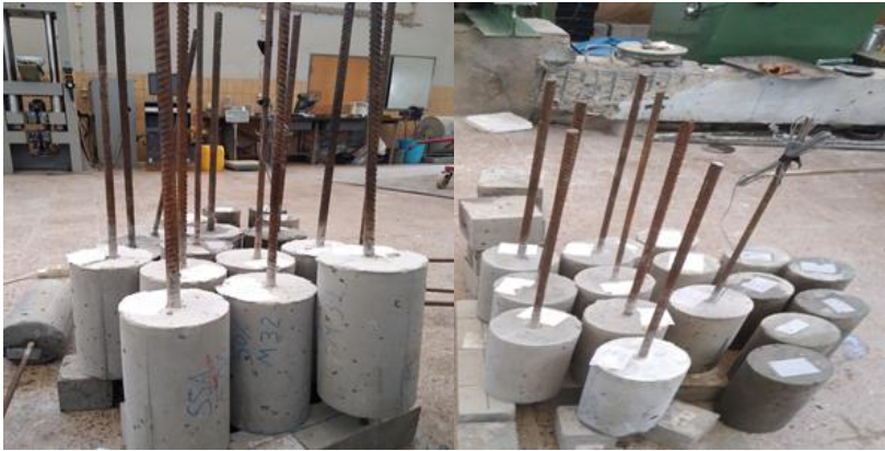
Figure 3.16. Specimens prepared for pullout test
