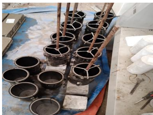
Figure 3.10. Oil smeared molds
