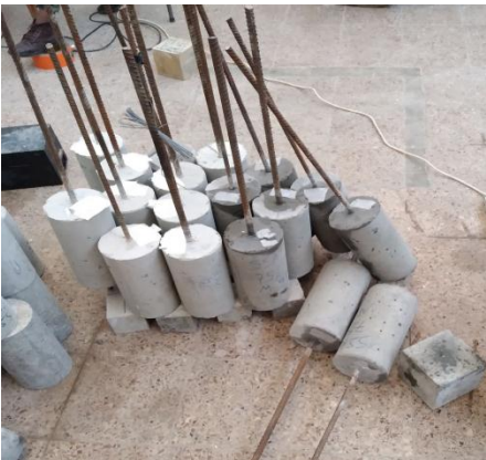
Specimens for pullout test
