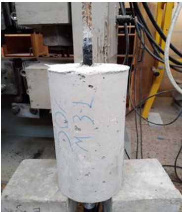
pullout Bond failure
