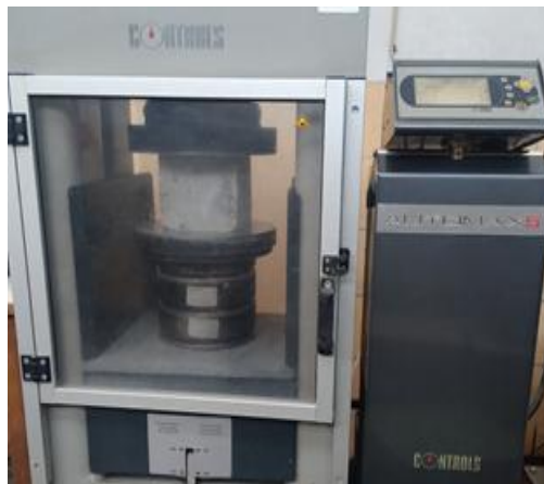
Figure 3.14. Test setup of Compressive strength test
