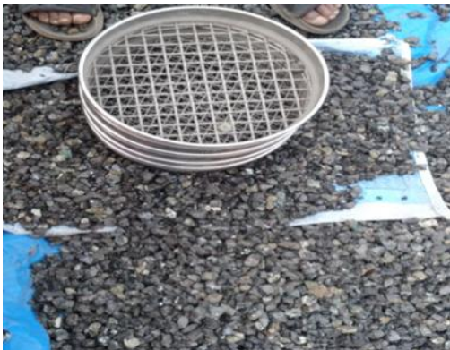
Sieving of steel slag aggregate
