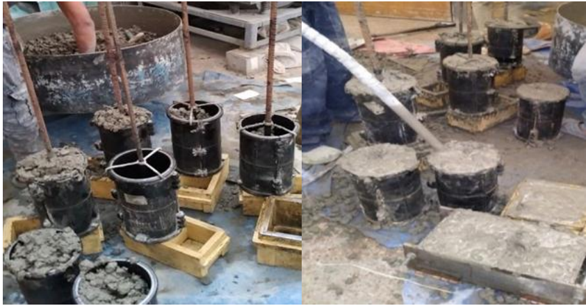
Figure 3.11. Casting and vibration of concrete
