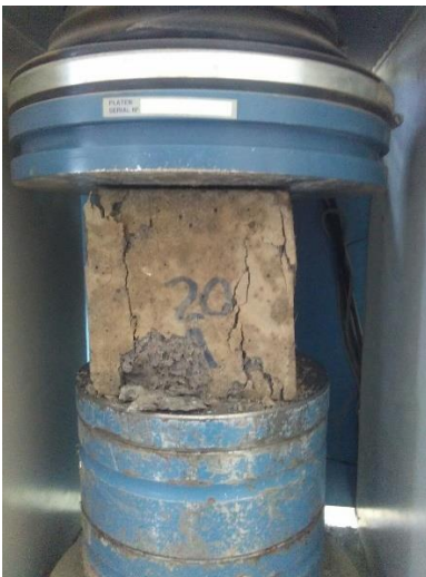
Compressive Strength Test and Shape of failed Cube
