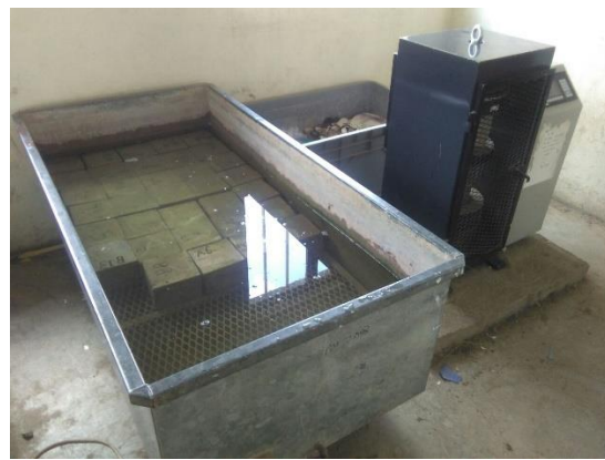
Bath for Concrete Cubes
