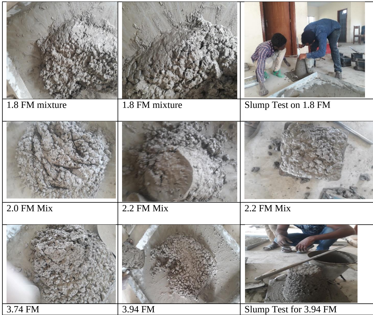
Figure 4. 6 Fresh Concrete Appearance for Different FM Values
