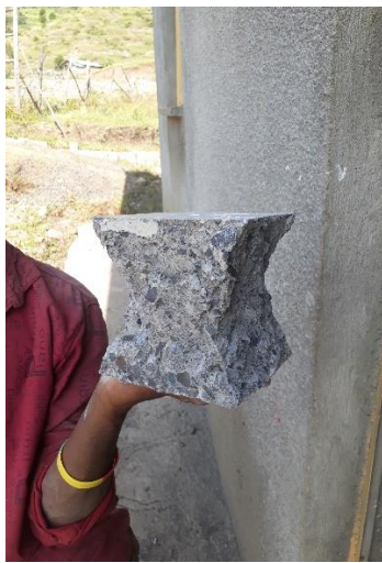
Compressive Strength Test and Shape of failed Cube
