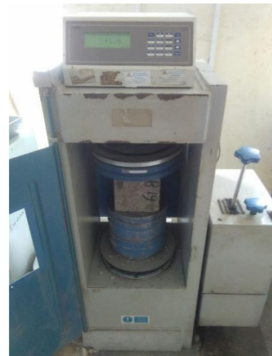
Compressive Strength Test and Shape of failed Cube
