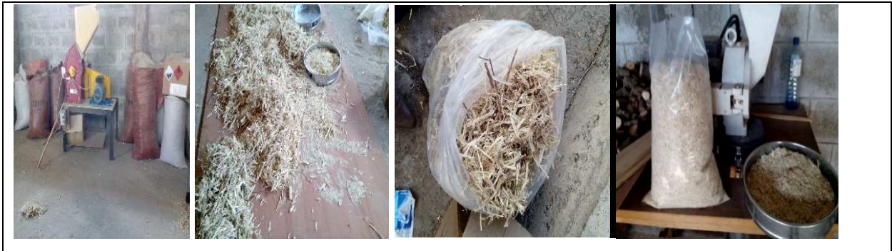
Figure 3-2 Experimental set up of size reduction process
