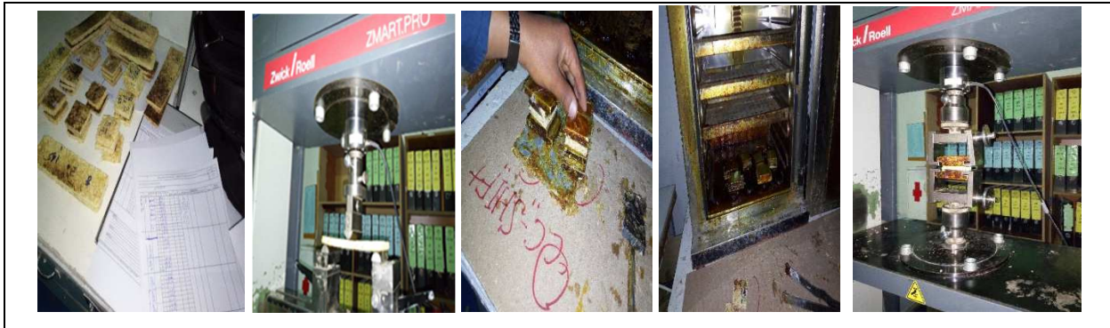
Figure 3-9 Experimental setup for bending strength and internal bonding test
