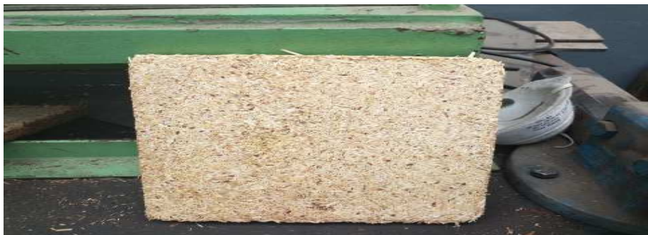
Figure 3-7 Final Trimmed board for test
