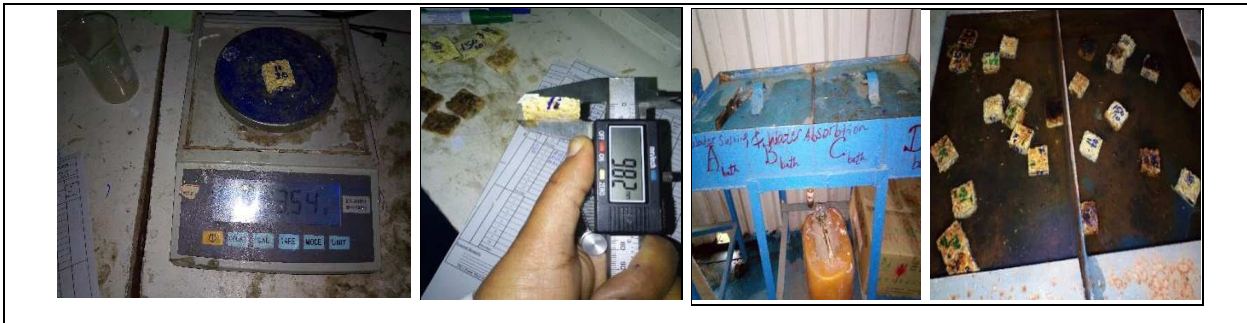
Figure 3-8 Experimental set up for (WA) and (TS) test
