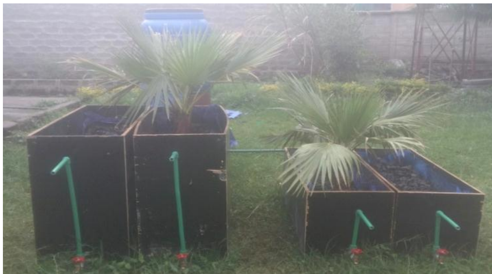
Figure 3-1: Pilot-scale HSSFCWs after plantation
