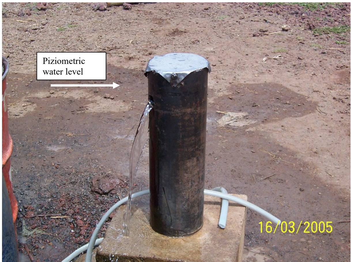
Plate 8.1. Artisan Well in Waliso town Borehole
