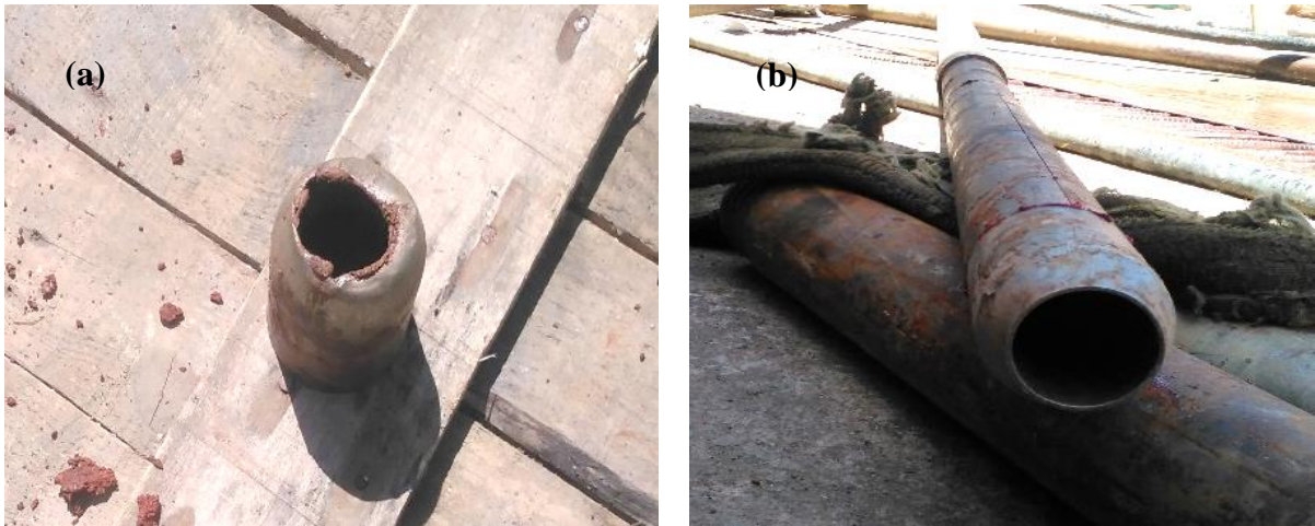
Plate 4.3 (a) Deformed driving shoe, (b) New driving shoe
