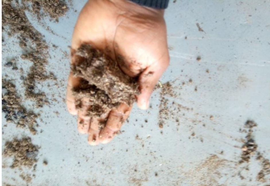
Figure 3.4 Crushed sample passing soil sieve 4.75mm.
