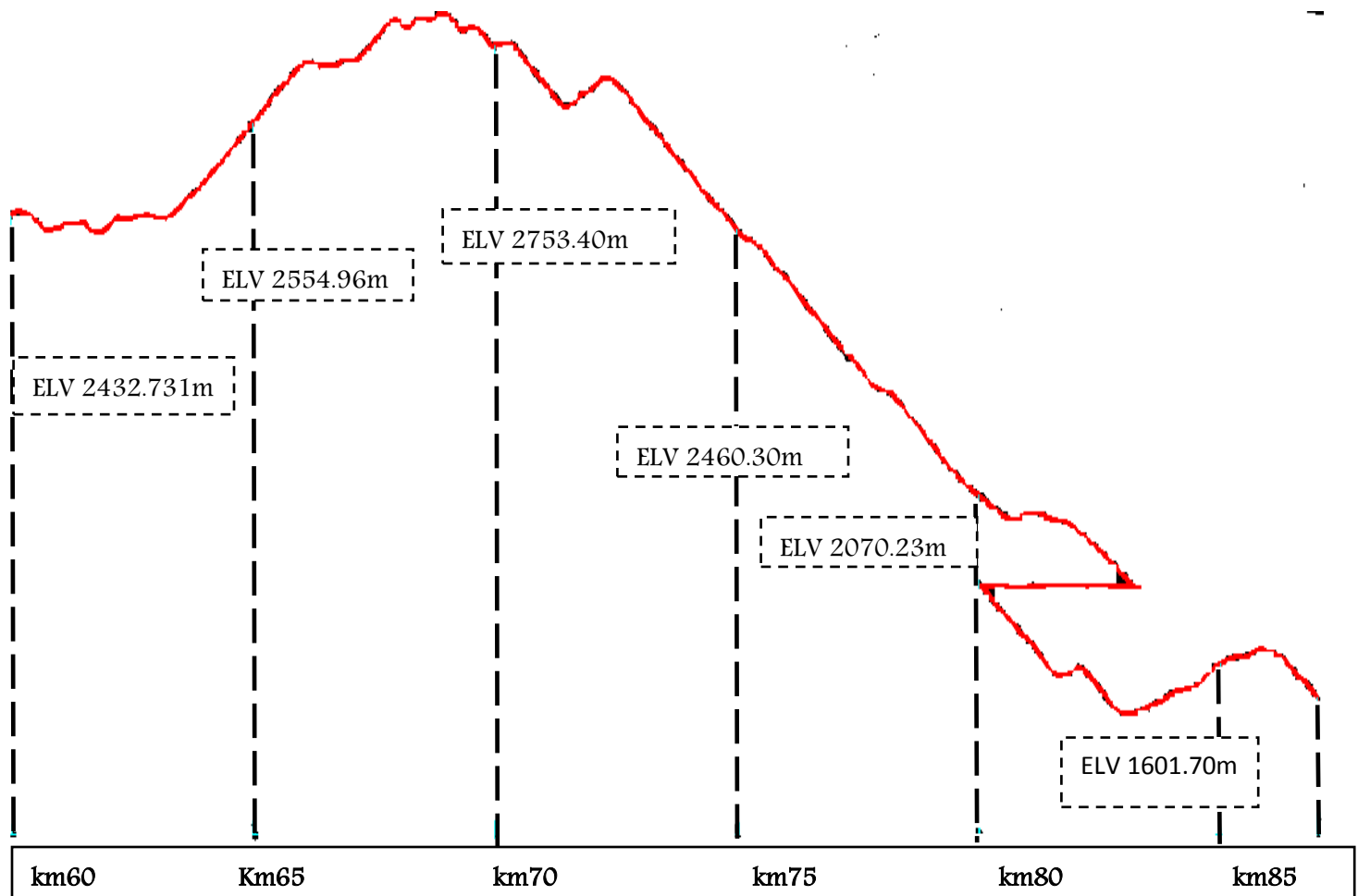
Figure 3.3: Vertical profile of designed road alignment
