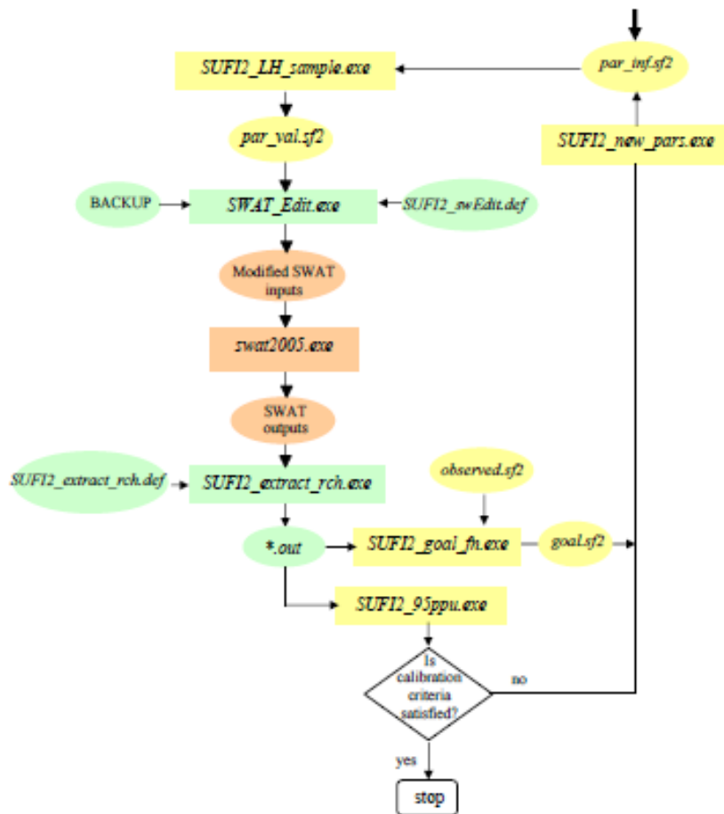
Figure 4-1: Link between SWAT (Orange), iSWAT (Green), and SUFI2 (Yellow) (Source: SWAT-CUP User Manual)
