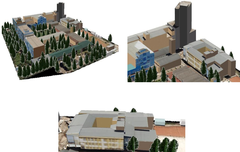
Figure 4.10. The LOD2 models are superimposed on the orthophoto: viewed at campus scale (top left), neighborhood-scale (top right), and building scale (bottom).
