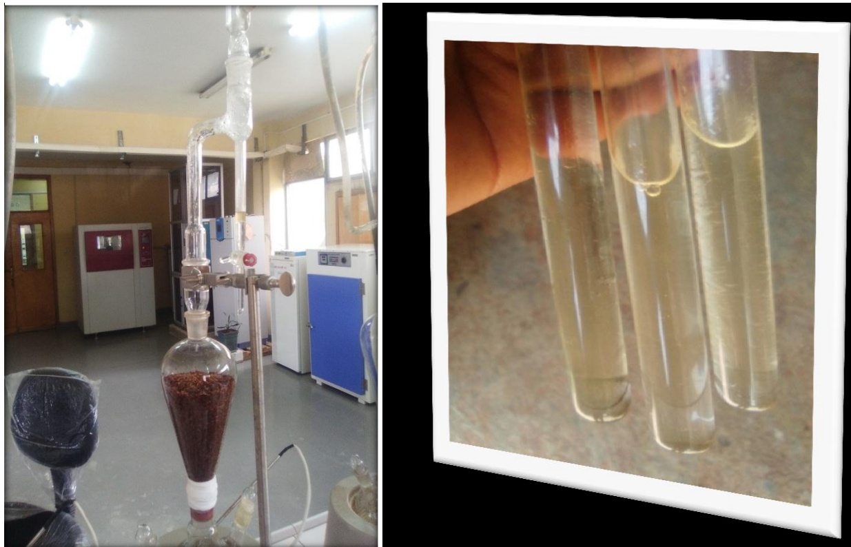
Figure C 3 :- steam distillation and juniper berries essential oil
