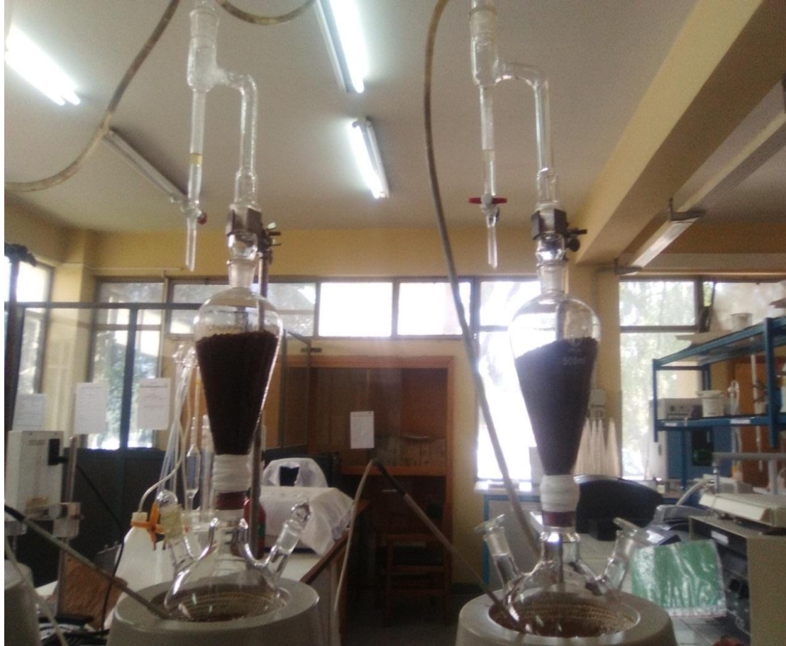
Figure 3.2 photograph of steam distillation equipment
