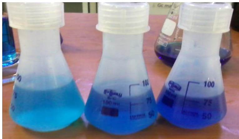
Picture C.5: Biochar absorption determination using Methylene Blue
