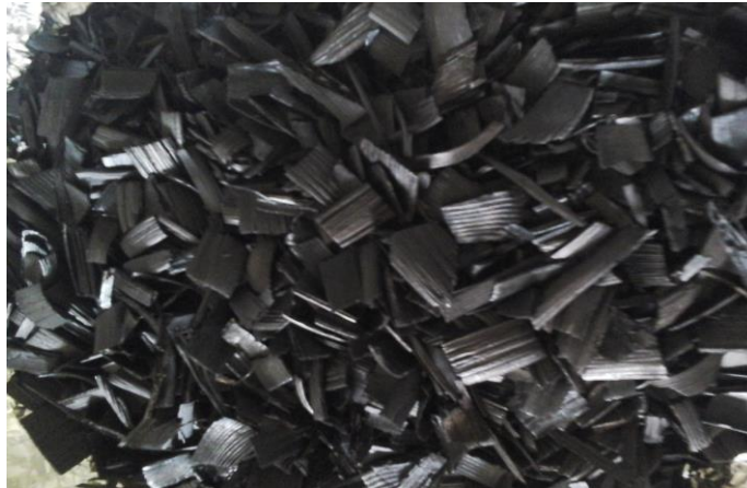
Picture C.1: Biochar produced through pyrolysis
