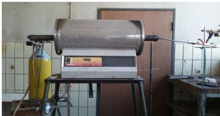
Picture C.3: Pyrolysis Equipment Setup
