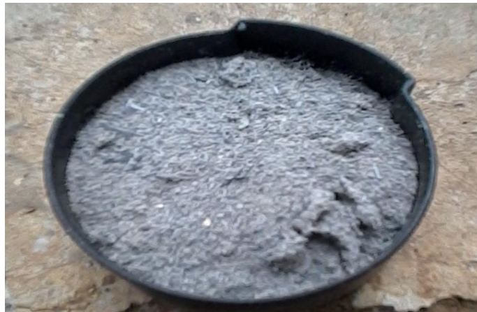
Picture C.2: Ash produced using muffle furnace
