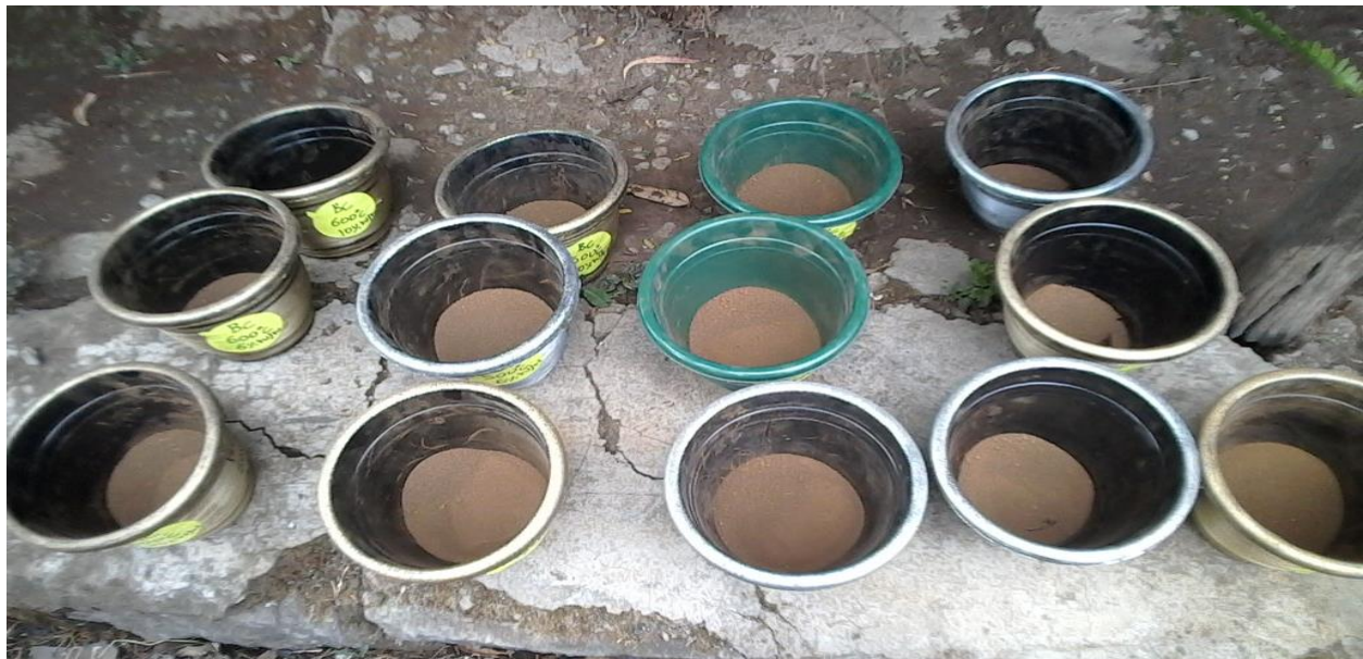
Picture C.4: Contaminated soil with remediation in incubation pots
