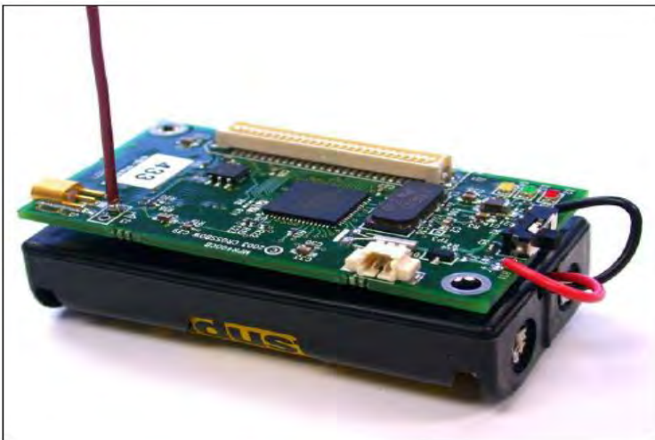
Figure 4.2 Mica2 Mote manufactured by Cross Bow Technology [30]
