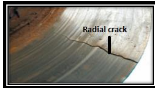
Figure 2 Actual photo of a premature failure of disc brake on Volvo B11R buss model
