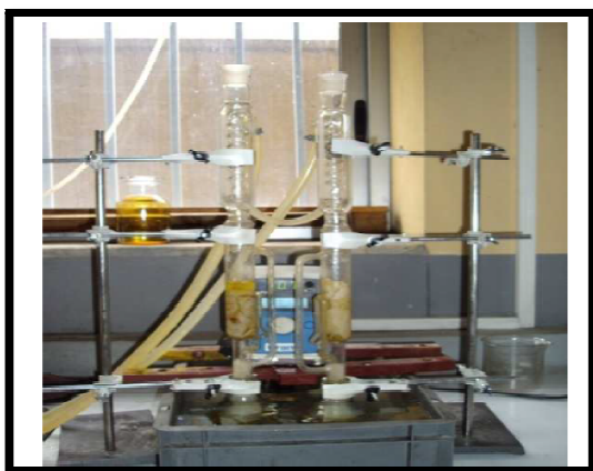
setting up soxhlet extractor together with the condenser.
