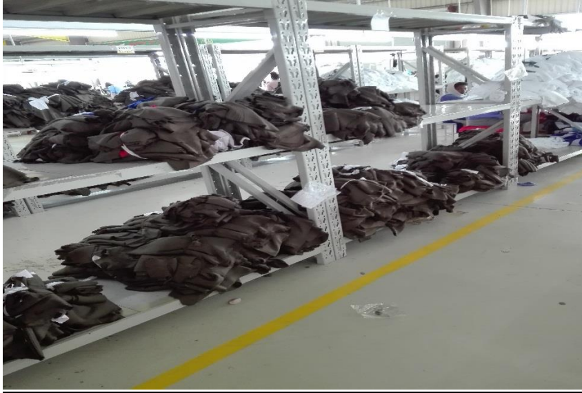
FIGURE 23: HIGH LEVEL OF INVENTORY ON CUTTING SECTION
