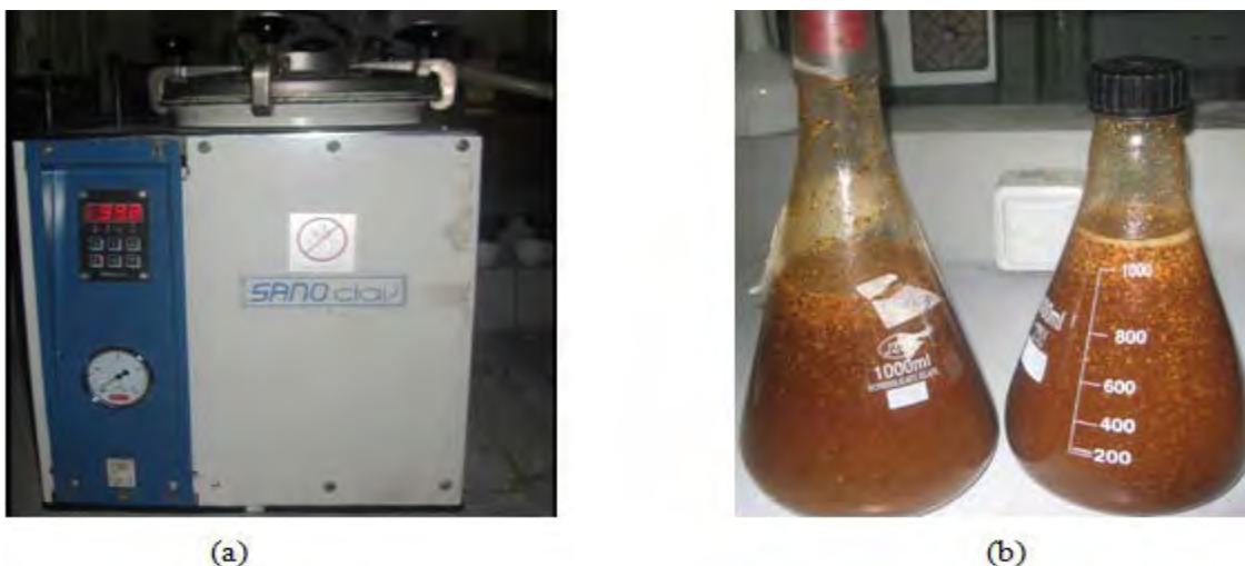
Figure 3.3 (a) Steam Pretreatment of fruit peels powder in autoclave (b) Sample ready for pretreatment
