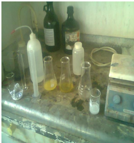
color change during titration for peroxide value
