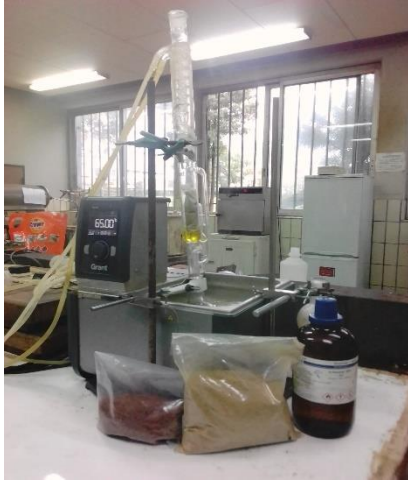
Laboratory setup for Brassica nigra seed oil extraction
