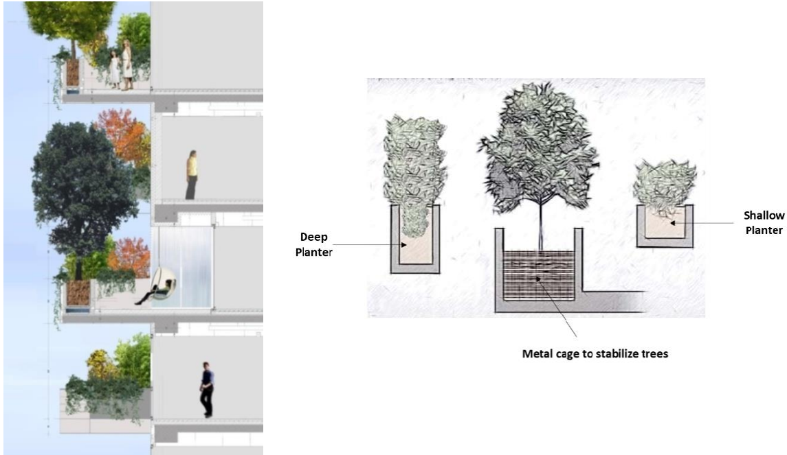
Figure 2.16 Sectional illustration and Planter detail of Bosco Vertical Building
