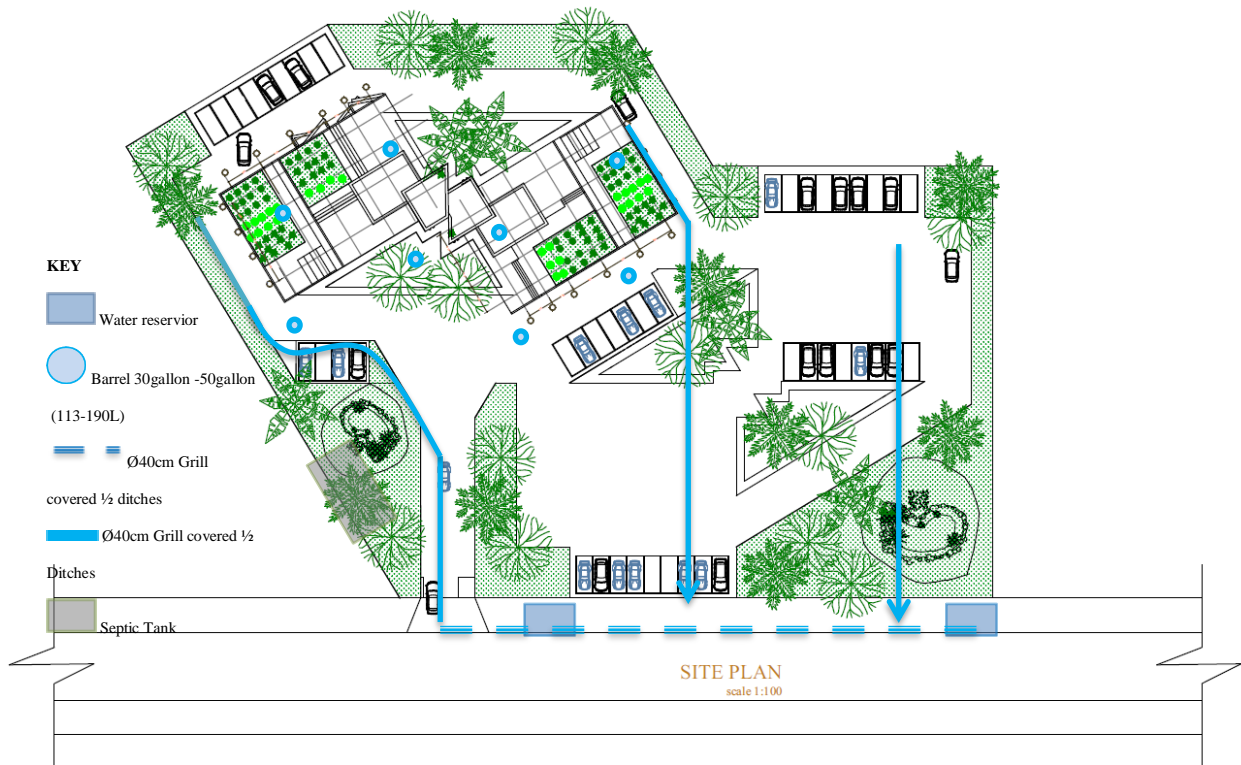
Figure 5.1 Surface an Rain Water Harvesting System
