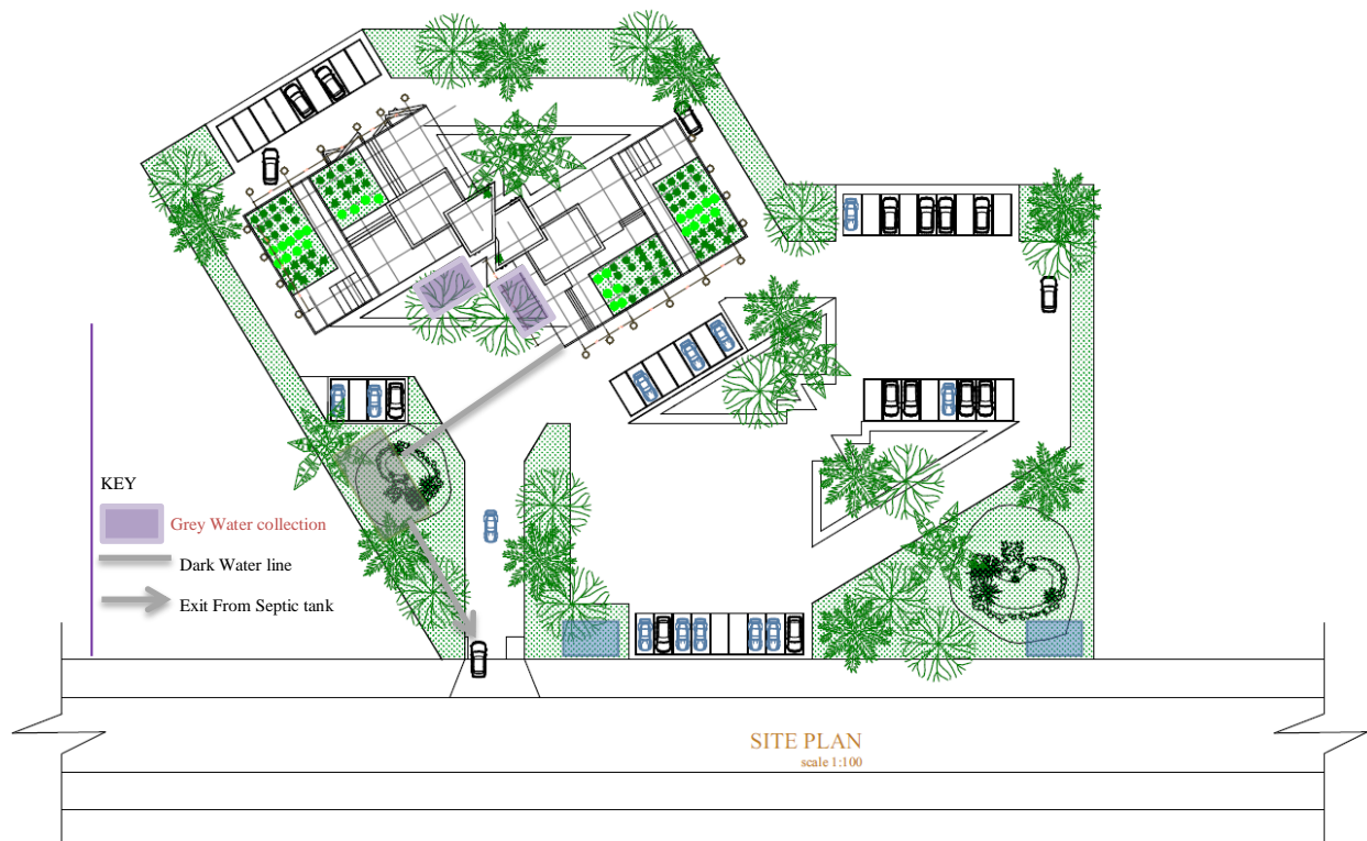
Figure 5.1 Sewage Drainage Systems
