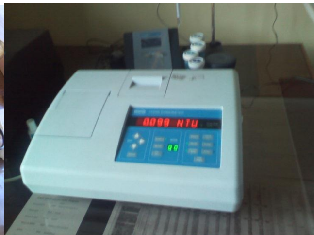
Figure 4-3: HACH 2100AN Turbidity meter
