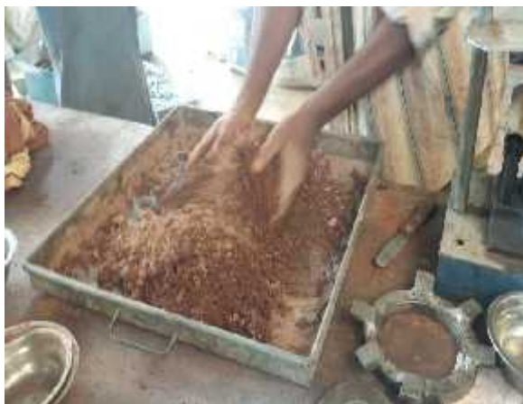
Picture 4-4 Preparation of Laterite-Cement Mixture
