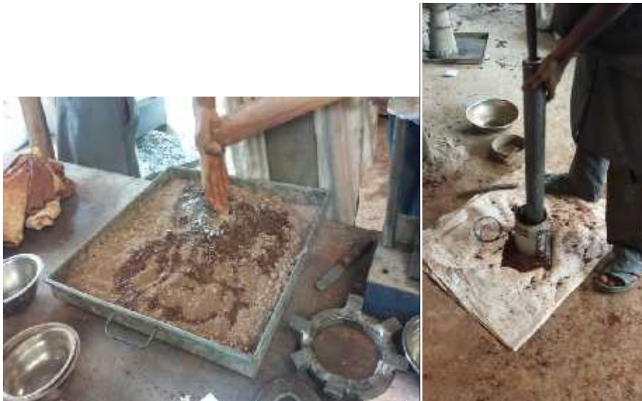
Picture 4-5 Moisture Density Test of the Laterite-Cement Mixture
