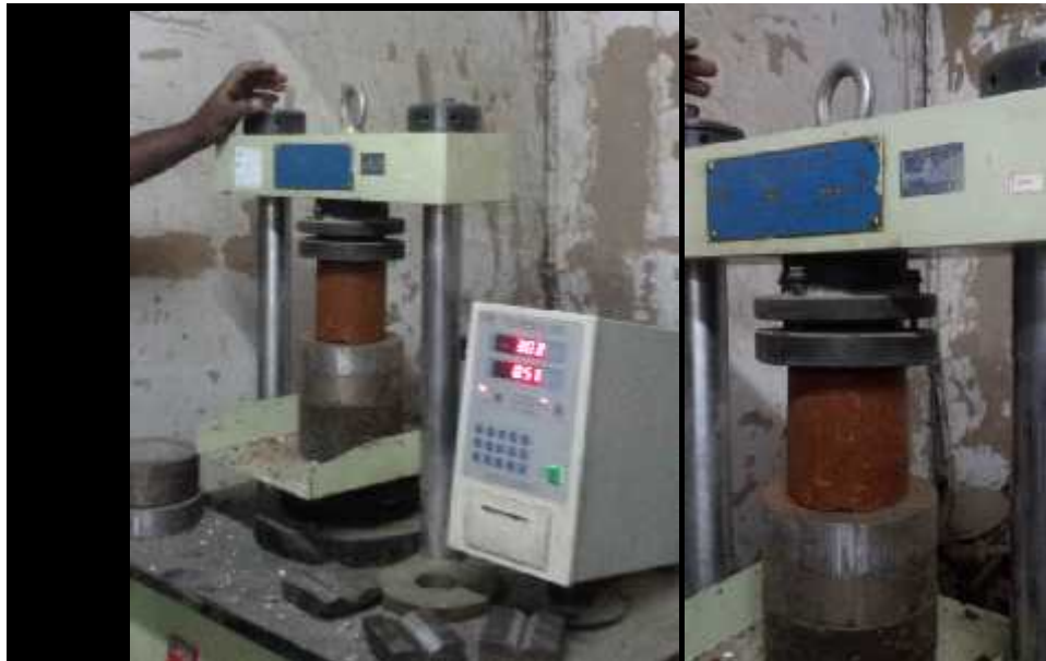
Picture 4-3 Unconfined Compression Test and Test Specimen Preparation
