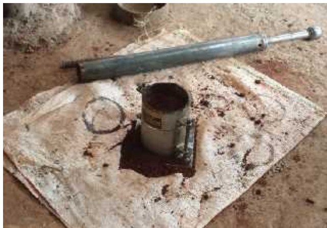
Picture 4-2 Moisture Density Test of the Lime-Laterite Mixture
