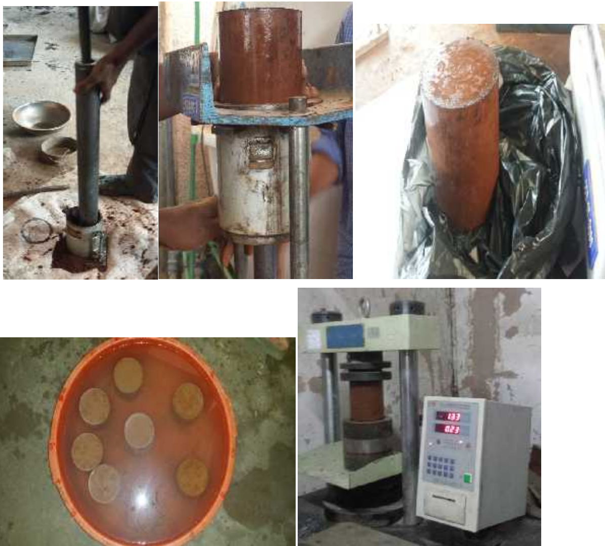
Picture 4-6 Unconfined Compression Test and Test Specimen Preparation
