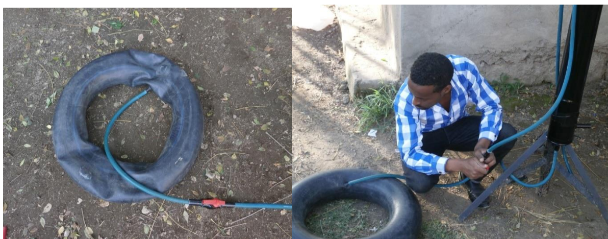
Figure 3. 6: Storing biomethane in to tyre tube
