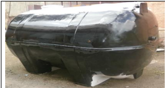
Fiber glass roto tanker (biogas digester)
