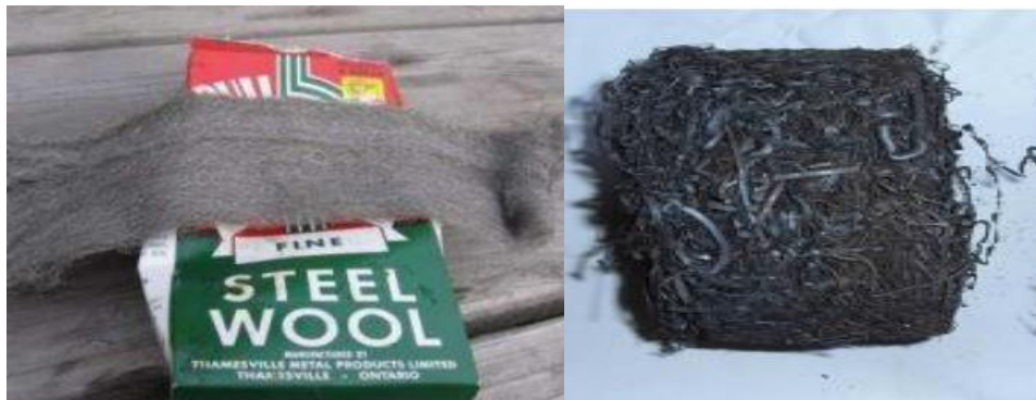
Figure 2. 3: Steel wool before and after H 2 S adsorption process[14].
