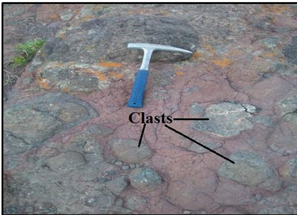
Fig.3.7: Field photograph of Agglomeratic basalt. Note coarse rounded to sub rounded shape clasts with a size of 1cm to 50cm (0557723E: 1415796N).
