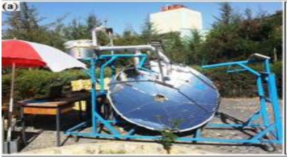
Figure 2.6 Indirect solar injera baking (Tesfay et al., 2019)
