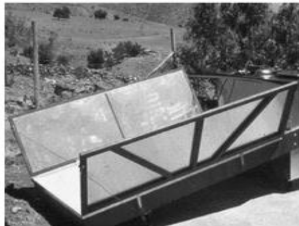
Figure 2.4 Indirect solar cookers: a flat-plate solar cooker (Schwarzer et al., 2003)
