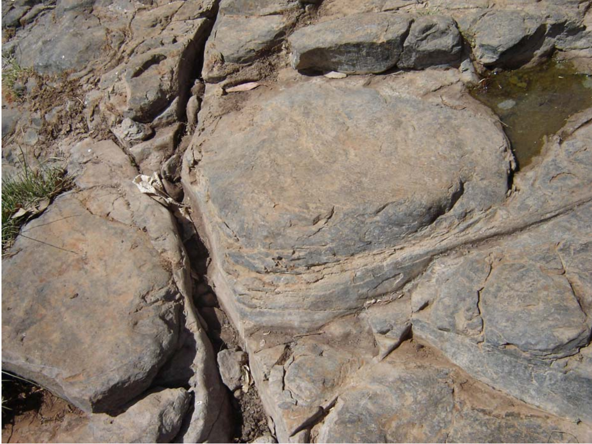
Figure 3.2 Spheroidal Weathering of Alaji basalt
