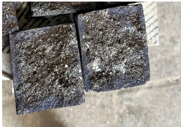
Figure 4.4 Change in colour of mortar specimen due to chloride attach
