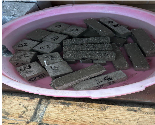
Pic4. curing of samples
