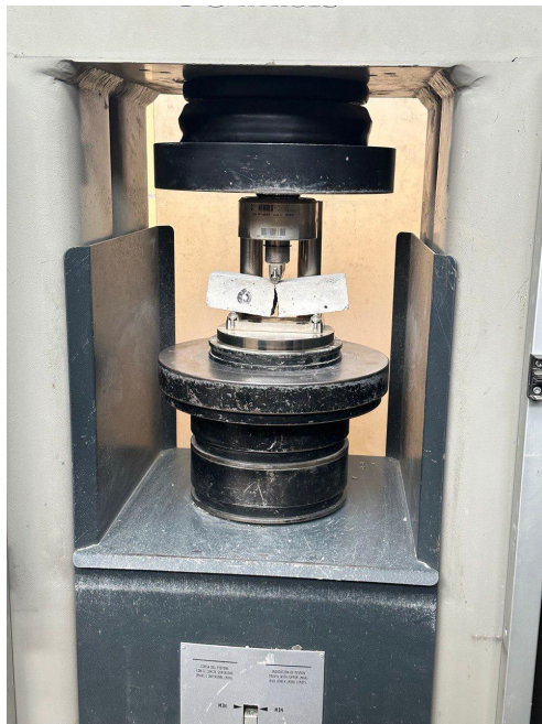
Pic 5. flexural and compressive strength tests
