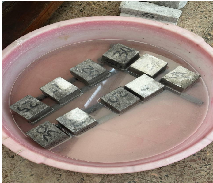
Pic 6. immersion of samples to salt and water solution for chloride penetration test
