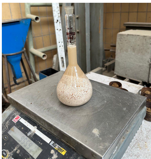
Pic3. photos taken while measuring the Specific Gravity of Egg shell and sand
