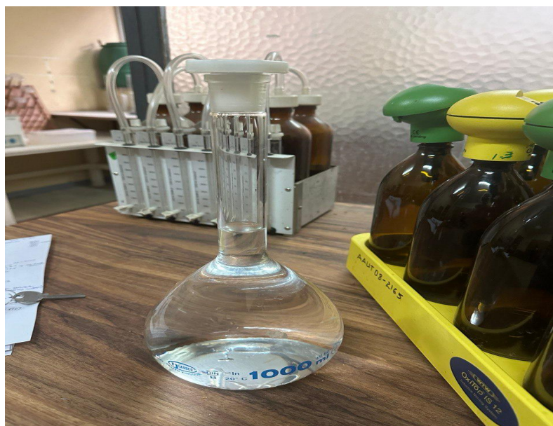
Pic 7. preparation of 0.1N silver nitrate solution for the determination of chloride penetration depth.
