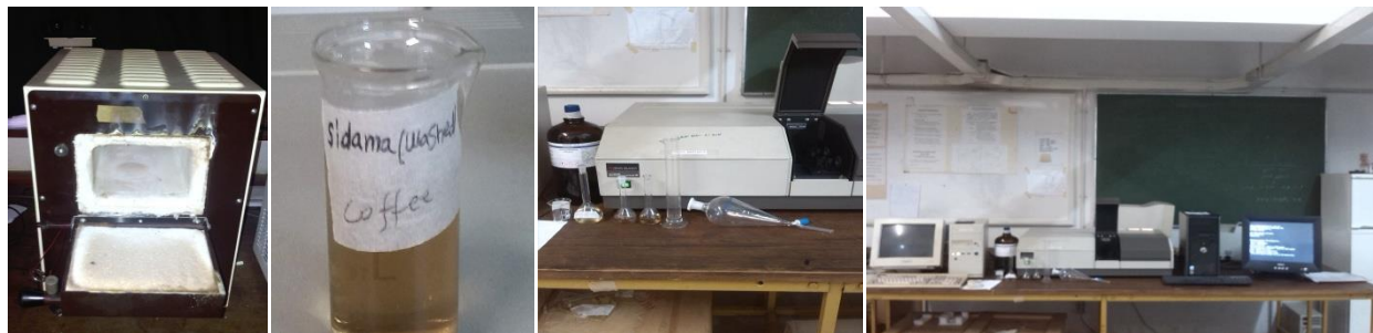
Fig 3.1:- Photograph of some experimental instruments used in UV/Vis absorption spectroscopy measurement of caffeine.
