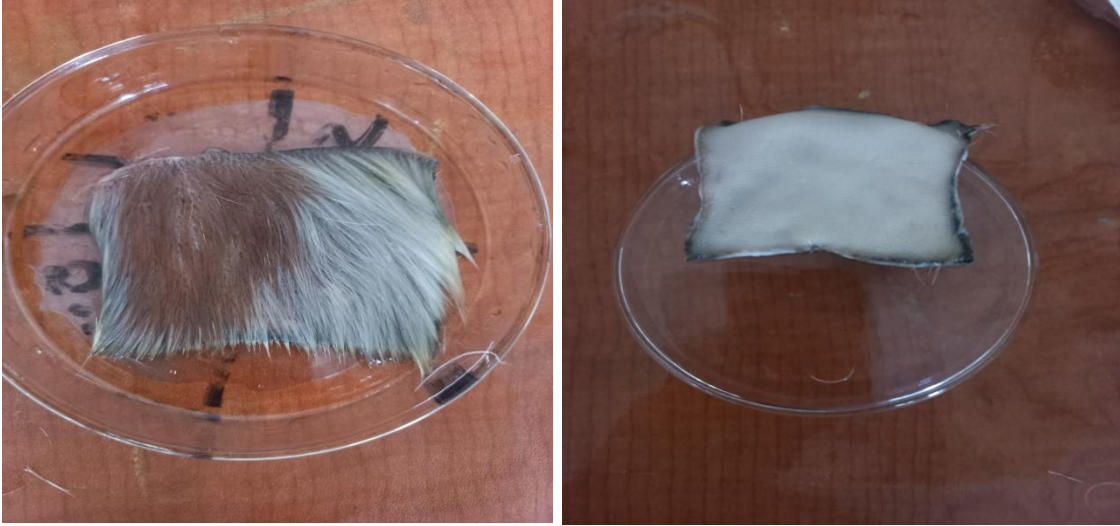
Figure 38 Pictures before and after dehairing
