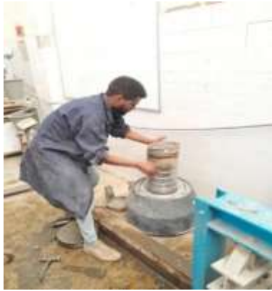
Figure3. 4.Sieving for graduation
