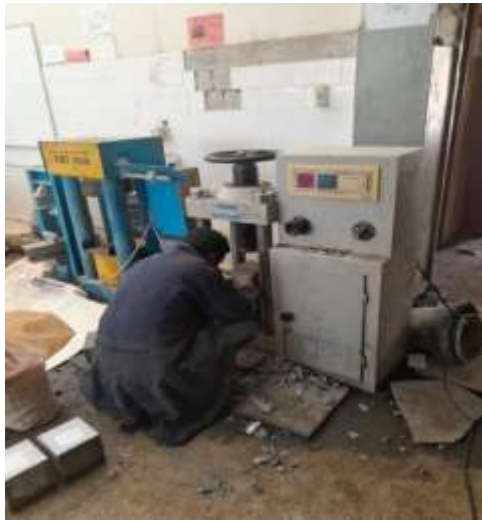
Figure3. 12.Compressive strength test
